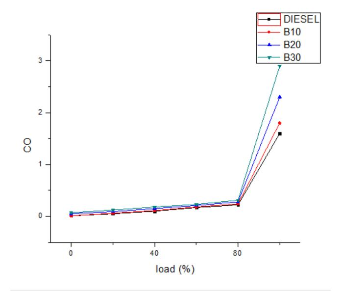
Vegetable oil contains larger value of oxygen than diesel, which acts as a combustion promoter in the cylinder. This results in better combustion than diesel. Hence CO ,which is due to incomplete combustion, is lower in these oils compared to diesel.
