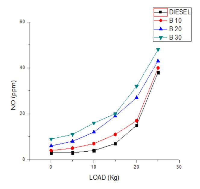
As vegetable oils have larger value of O<sub>2</sub> than diesel so oil burns more inside the cylinder which leads larger value of temperature inside the cylinder which is the main cause of the larger value of NOx.
