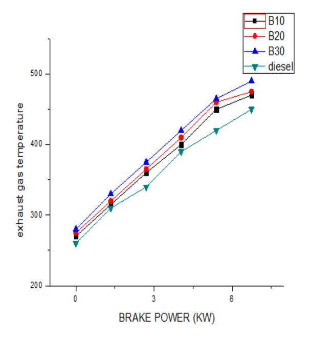
Exhaust gas temperature in case of diesel is the lowest compared to other blending.
