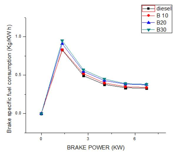
Brake specific Fuel consumption in case of pure diesel is the lowest than 10,20 and 30% blending.
