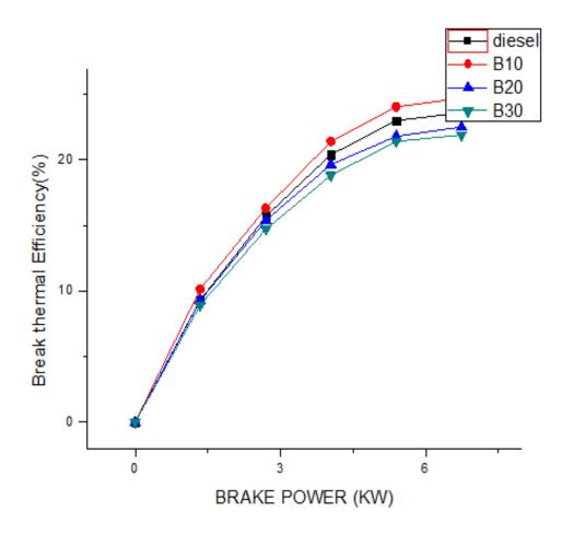
Break thermal efficiency in case of blending 10% is highest in comparison to 20% blending,30% blending and pure diesel. We get optimum value in case of 10% blending.
